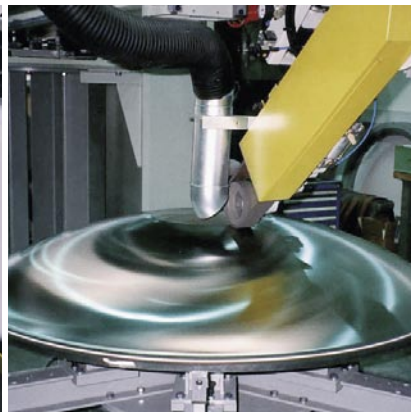
External grinding of ends
